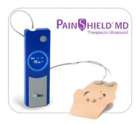
The driver's approximate dimensions are  $39 \times 12 \times 125$  mm (or  $1.5" \times 7/16" \times 47/8"$ ). The patch weighs about 10g (or 0.4 oz.) and its dimensions are 120 mm x 70 mm (or 4  $10/16" \times 25/8"$ )
